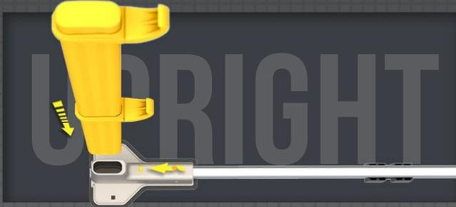
Put handrail and kneerail onto tube fixing then fix them by tightening screw
