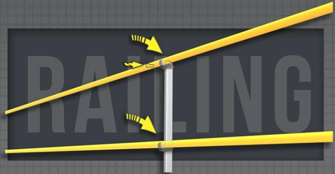
Use tube junction to extend the railing, once the tube and junction get connected, fixed tube to junction by tekscrew
